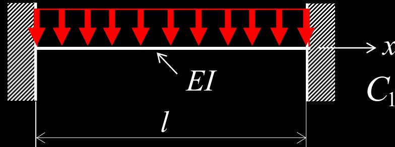
$$v(x) = \frac{wl^4}{24EI} \left\{ \left(\frac{x}{l}\right)^4 - 2\left(\frac{x}{l}\right)^3 + \left(\frac{x}{l}\right)^2 \right\}$$
