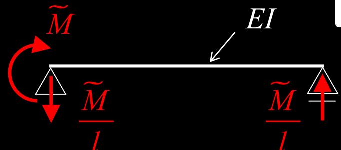
$$\left\{ \begin{array}{l} C_1 = \frac{\tilde{M}}{l}, C_2 = -\frac{\tilde{M}}{l}, \\ C_3 = \frac{1}{3} \frac{\tilde{M}}{l}, C_4 = 0 \end{array} \right.$$
