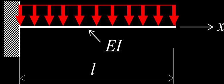
$$v(x) = \frac{wl^4}{24EI} \left\{ \left(\frac{x}{l}\right)^4 - 4\left(\frac{x}{l}\right)^3 + 6\left(\frac{x}{l}\right)^2 \right\}$$
