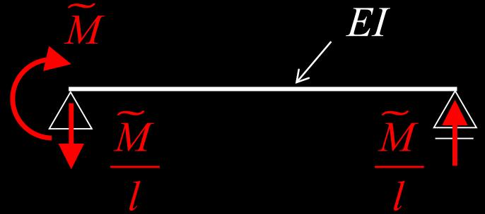
$$\begin{aligned}EIv^{IV}(x) &= 0 \\ EIv'''(x) &= C_1 \\ EIv''(x) &= C_1x + lC_2\end{aligned}$$
