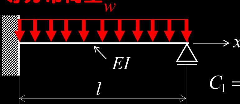
$$C_1 = -\frac{5}{8}, C_2 = \frac{1}{8}, C_3 = C_4 = 0$$
